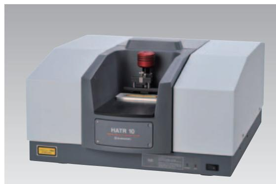
Fig. 2 IRAffinity-1 Unit with HATR10 Attachment Installed
