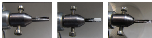
Figure 1: A high purity tantalum sample holder (left) acts as an electrode in the analysis of alumina powder (center) and sapphire wafer (right).
